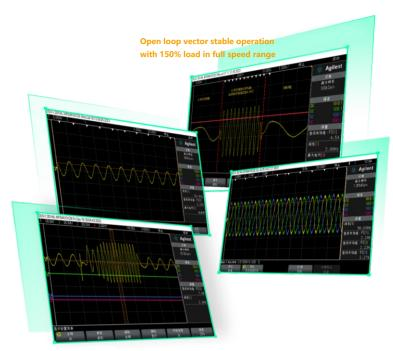
New high-performance vt control algorithm, stable operation at 0.1Hz with 150% load
