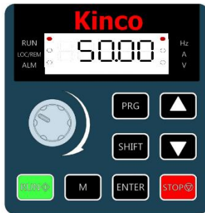
Figure 4-7 Steady operation display of the AC drive
