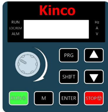
Figure 4-1 Schematic diagram of the LED operating panel
