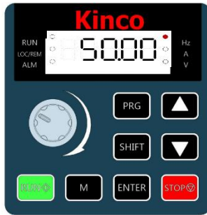
Figure 4-6 AC drive power-on display
