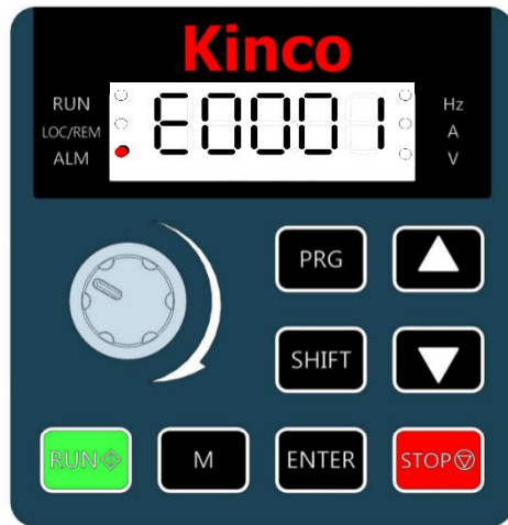
Figure 6-1 The interface fault display
